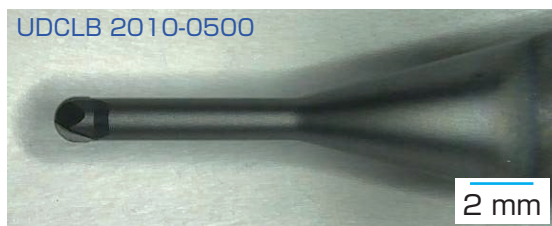
Tool #2 milled 131.9 \text{ mm}^3 in 76.5 minutes.
