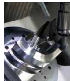
外壁曲面仕上げ・大R隅取り Outer curved wall finishing Large R corner finishing
