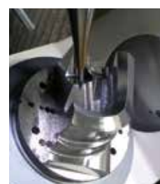
内壁曲面仕上げ Inner curved wall finishing
